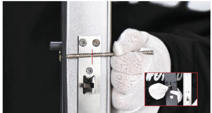
12. Pass the bamboo-shaped screw through the rear lock gasket. Trim the bamboo-shaped screw length according to the door thickness so that it does not exceed the outdoor door edge. Make a mark.
