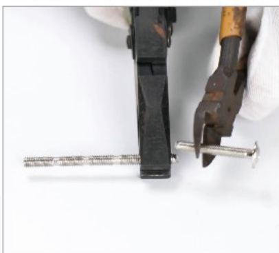
13. Use pliers to cut off the marked bamboo-shaped screw
